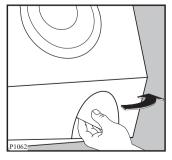
Release the emergency emptying hose, place it in the container, and remove its cap by unscrewing it.
